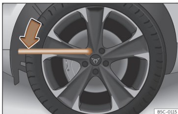
Fig. 209 Tyre change: slacken the wheel bolts.
