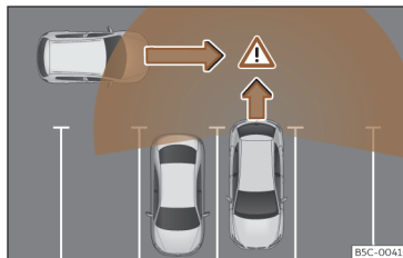
Fig. 143 Diagram of the parking assistant: detected area around the vehicle that is driving off.
