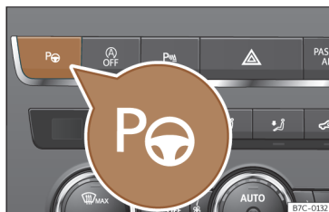
Fig. 131 In the centre console, top section: button to switch on the Park Assist system.
