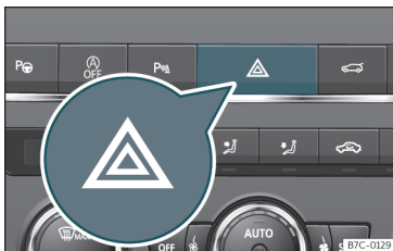
Fig. 95 Dash panel: hazard warning lights switch
