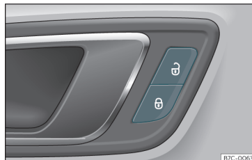
Fig. 75 Driver's door: central locking switch.
