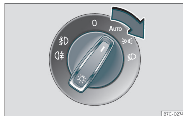
Fig. 92 Dash panel: lights control.
