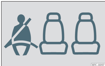
Fig. 5 Instrument panel: left rear seat occupied and corresponding seat belt fastened display.
