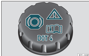
Fig. 206 Engine compartment: brake fluid reservoir cap.
