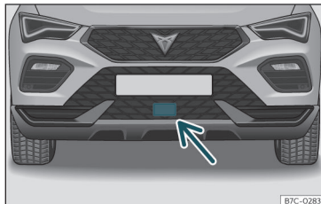
Fig. 148 On the front bumper: radar sensors.
