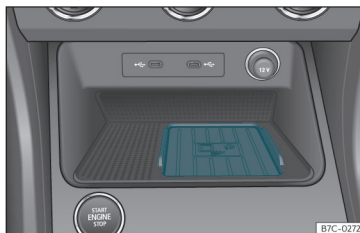
Fig. 136 In the centre console: pad for the mobile phone connection.
