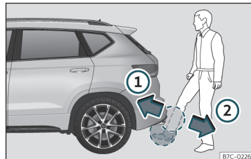
Fig. 85 Rear lid with sensor-controlled opening (Easy Open).
