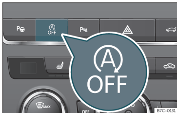
Fig. 141 Centre console: Start-stop system button.
