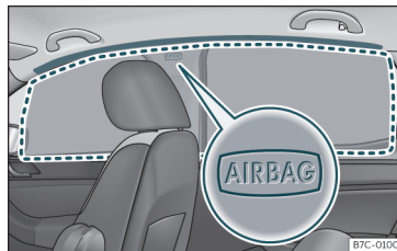
Fig. 21 Location of head-protection airbags.
