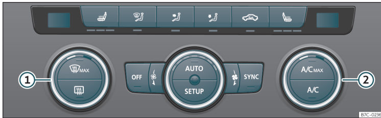
Fig. 129 In the centre console: Climatronic controls.
