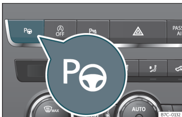
Fig. 177 In the upper part of the centre console: button to switch on the Park Assist system.
