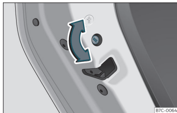
Fig. 81 Childproof lock on the left hand side door.
