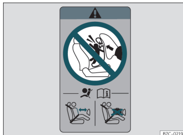
Fig. 24 Airbag sticker: on the rear frame of the passenger side door
