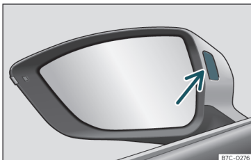
Fig. 170 Control lamp of the lane departure warning.
