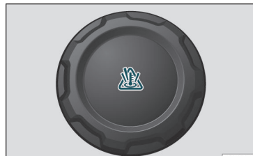
Fig. 205 Engine compartment: coolant expansion tank cap.
