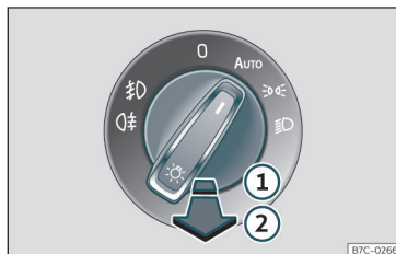
Fig. 93 Dash panel: lights control.
