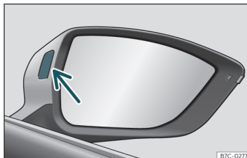
Fig. 171 Control lamp of the lane departure warning.
