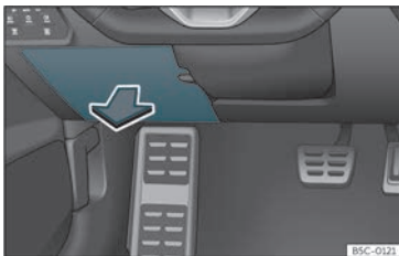
Fig. 47 On the driver's side dashboard: fuse box cover.
