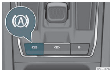
Fig. 176 In the lower part of the centre console: Auto Hold function button.
