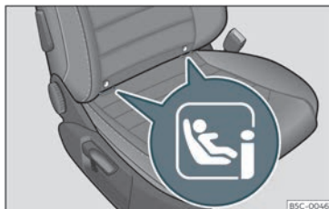
Fig. 28 Front passenger seat: ISOFIX/i-Size securing rings.
