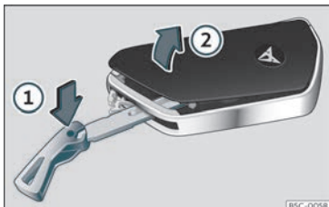
Fig. 72 Vehicle key: opening the battery compartment cover.
