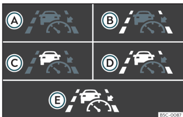
Fig. 166 On the instrument panel display: control lamps.
