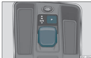
Fig. 145 In the centre console: selector lever.
