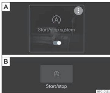
Fig. 144 On the Infotainment system screen.: Start-Stop system connected. A ) View in the main menu. B ) View with the Infotainment system off.
