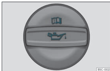
Fig. 205 In the engine compartment: Engine oil filler cap.
