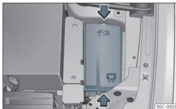
Fig. 48 In the engine compartment: fuse box cover.
