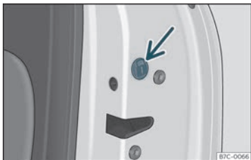
Fig. 79 Locking the door manually.
