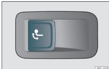
Fig. 187 On the left side of the luggage compartment: button for unlocking the tow hook.
