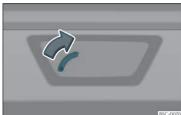
Fig. 85 Detail of the luggage compartment: emergency unlocking
