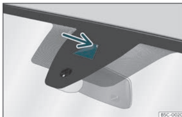
Fig. 150 On the windscreen: field of vision of the Lane Assist system.
