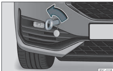
Fig. 44 Right side of the front bumper: towline anchorage in position.
