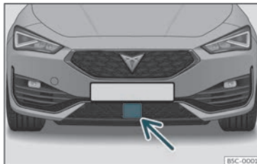
Fig. 148 On the front bumper: radar sensors.
