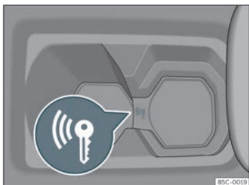
Fig. 143 In the centre console: emergency start.
