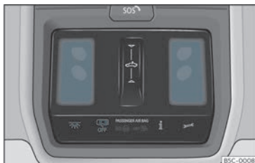
Fig. 92 Detail of roof lining: front lighting of the passenger compartment.
