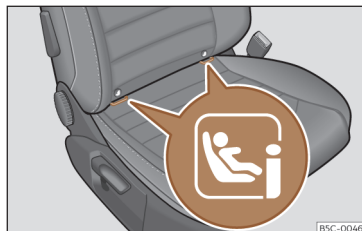
Fig. 32 Front passenger seat: ISOFIX/i-Size securing rings.
