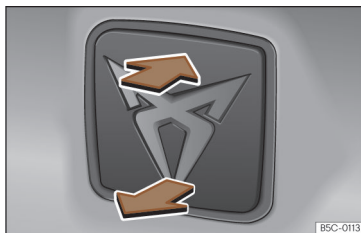
Fig. 87 Rear lid: opening from outside.
