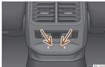
Fig. 155 Rear part of the centre console: USB connectors with power outlet function.
