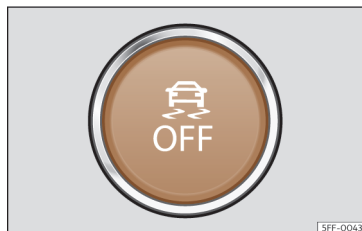
Fig. 191 In the lower part of the centre console: button to switch the ESC off/on
