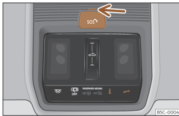
Fig. 36 On the roof console: voice service controls
