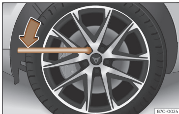
Fig. 42 Wheel change: loosen the wheel nuts.
