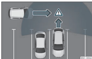
Fig. 183 Schematic representation of the rear cross traffic alert assistant: zone monitored around the vehicle while leaving a parking space.
