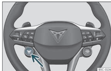
Fig 158 Multifunction steering wheel*: button to change the driving profile.
