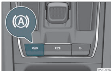
Fig. 187 In the lower part of the centre console: Auto Hold function button.
