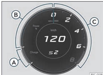
Fig. 61 Digital instrument panel: Powermeter (Cupra view)
