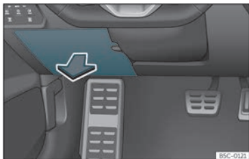
Fig. 51 On the driver's side dashboard: fuse box cover.
