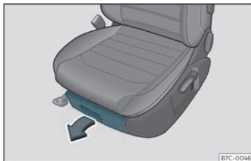
Fig. 138 Storage compartment under the front seats.
