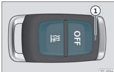
Fig. 144 Auxiliary heating: radio-operated remote control.
