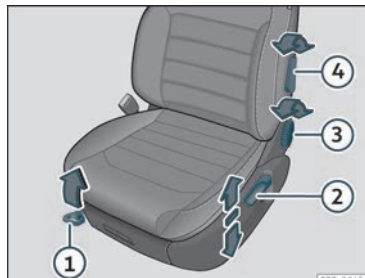
Fig. 104 Front seats: manual seat settings.
