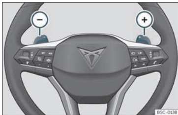
Fig. 157 Steering wheel: automatic transmission levers
