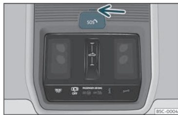
Fig. 36 On the roof console: voice service controls
