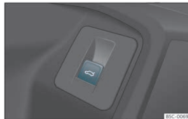
Fig. 87 On the driver's door: button to open and close the rear lid.
