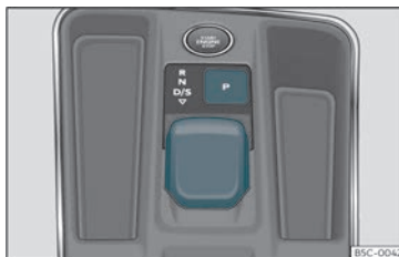
Fig. 156 In the centre console: selector lever.
