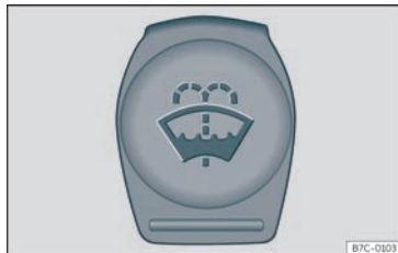
Fig. 220 In the engine compartment: window washer tank cap.
