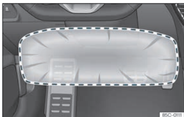
Fig. 22 On the driver side: airbag action radius for the knees.
