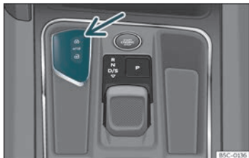
Fig. 74 Centre console: vehicle key socket.
