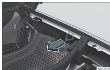
Fig. 205 Between the left wing panel and the engine bonnet hinge: Charging connector manual release mechanism puller.
