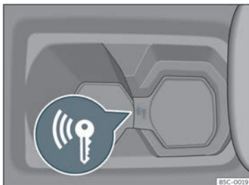
Fig. 154 In the centre console: emergency start.
