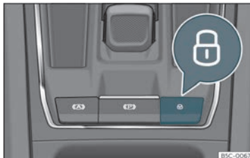
Fig. 79 In the centre console: central locking switch
