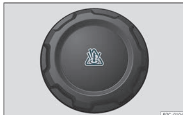
Fig. 218 Engine compartment: coolant expansion tank cap.
