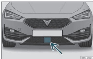
Fig. 159 On the front bumper: radar sensors.
