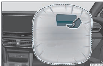
Fig. 18 Front passenger airbag located in instrument panel.
