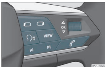
Fig. 64 Right side of the multifunction steering wheel: buttons for using the instrument cluster's menus and information displays (depending on versions).
