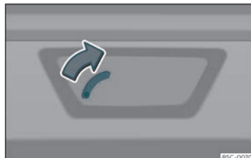
Fig. 90 Detail of the luggage compartment: manual release mechanism (Leon Sportstourer).
