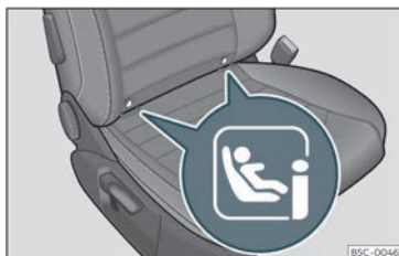
Fig. 32 Front passenger seat: ISO-FIX/i-Size securing rings.
