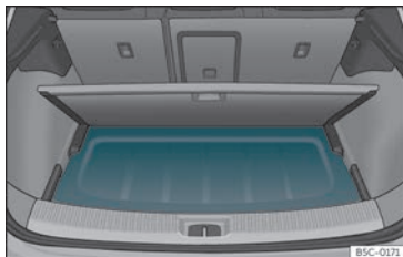
Fig. 117 In the luggage compartment: fitting the rear shelf.
