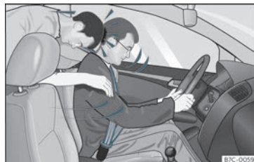
Fig. 12 The unbelted passenger in the rear seat is thrown forward violently, hitting the driver who is wearing a seat belt.
